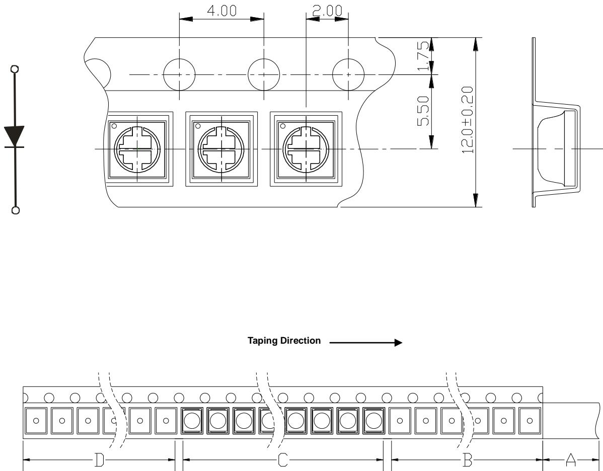
A: Top Cover Tape, 300mm; B: Leader, Empty, 200mm; C: 1000 Lamps Loaded; D: Trailer, Empty, 200mm.
